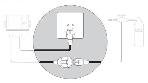
Remote sensor kit with 5 meters cable can be used to monitor co2 concentration in confined space.
