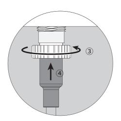
Firmly connect the port ① into the port ②, then push ③ and rotate ④ the middle metal part in the direction shown.
