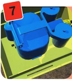
Once you have connected the AQUAvalve to the 6mm pipe, simply pull the pipe back through so that all the excess pipe inside the AQUAbox is pulled out. As you pull the pipe out lower the AQUAvalve so that it locates onto the Tee section in the AQUAbox.
