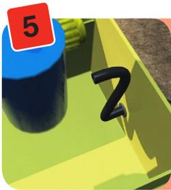
Take the 2 meter length of 6mm pipe and push it, (from the outside) through the 6mm Top Hat Grommet, as shown in the image. Pull the pipe through the grommet so that there is approximately 150mm inside the AQUAbox.
