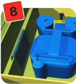
Once you are happy that the AQUAvalve is connected to the AQUAbox and all the excess pipe has been pulled out. Then take your 2 pieces of Tee shaped capillary matting.
