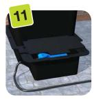
11.1 Place the black lid over the AQUAvalve. So the lid can be easily removed place it so that the 4 studs are facing upwards. For the first few weeks after the tank is filled and the AQUAvalve is working you can leave the black lid off so that you are happy that the AQUAvalve is flooding & draining correctly.
